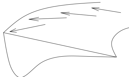
Fig. 3: Impinging flow in channel bends
